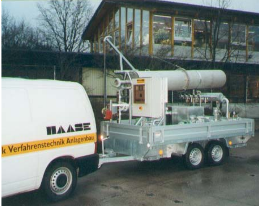
Mobile booster unit with flare
